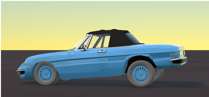
Figure 41. Example of agent full braking making the car tilt forward due to inertia.
